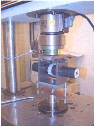
Fig. 2: Fatigue test in the testing machine Instron, sample 1.
