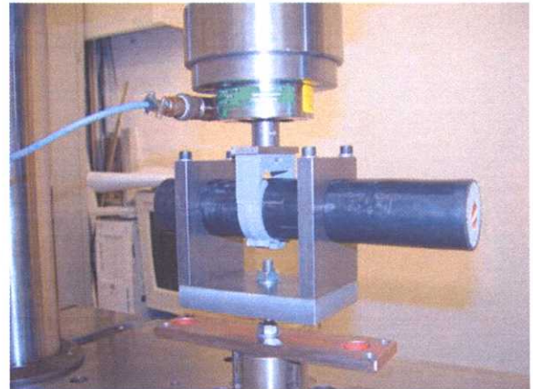
Fig. 3: Fatigue test, pipe clamp shifted by 90°, in the testing machine Instron, sample 2.
