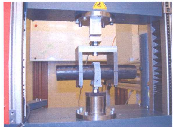
Fig. 5: Static rupture test, test machine Zwick, with previous fatigue, sample 1.
